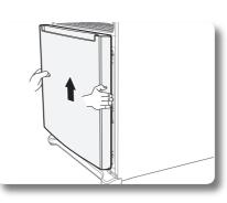
Remove the Freezer door by lifting it upward.
